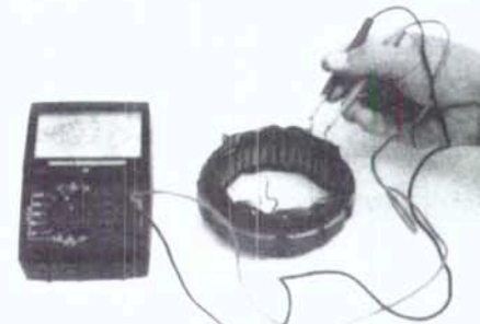
Fig. 77—Check stator coil leads for continuity.
